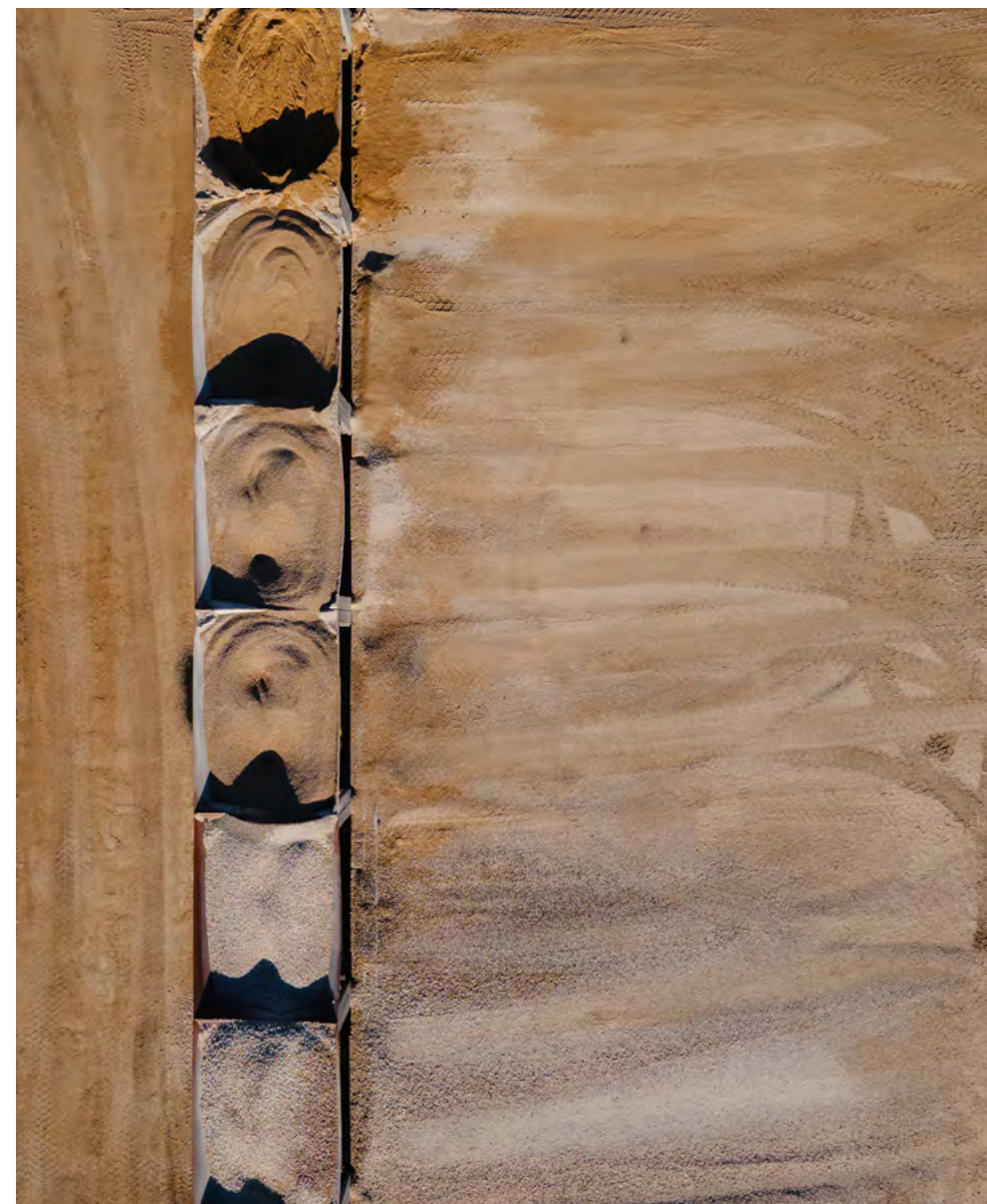
Cold feed bins at a Gulf Coast plant in Houston, Texas, United States. Gulf Coast is part of the Texas Region in CRH's Americas Materials Division and provides asphalt/paving, construction services, industrial and builder's products to the Southeast Texas region's growing economy.
