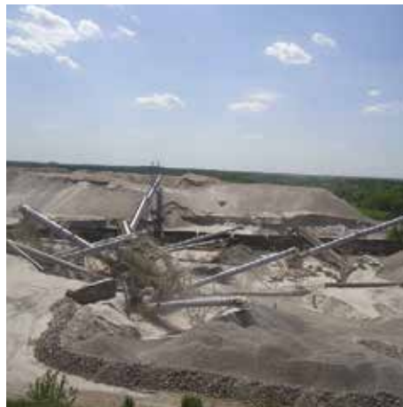
A modern crushing and screening plant was installed at Bekhy Quarry in Ukraine during 2015. The new fully automated plant has increased the quarry's production capability and significantly improved its environmental standards while reducing specific energy consumption.
