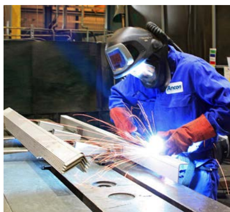
Metal Inert Gas (MIG) welding of a stainless steel brick cladding support system at Ancon's 6,500m 2 manufacturing facility in Sheffield, UK. Ancon, part of Europe Lightside, is a two-time winner of the Queen's Award for Enterprise.
